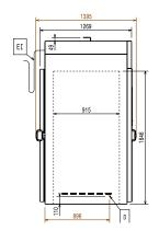
Drain Electrical inlet (power) ΕI Refrigerant Outlet
